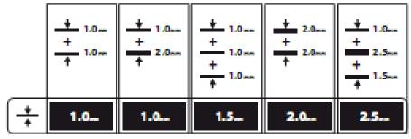
**2 - Mode B:** Welding with the clamp in manual mode (intensity and duration of welding shall be selected) *Intensity and time adjustment table:*
